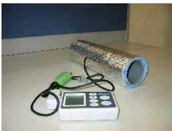
Fig.2 Observation probe (a temp-hygro sensor with data logger)
